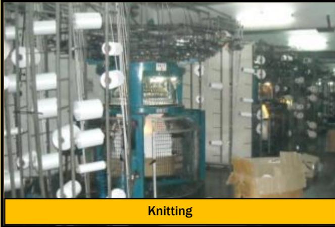
Knitting is also carried out in circular knitting machine where there is no requirement of weft inserting shuttles or jets across warp. The process is a loop forming techniques using couple of hundred of metallic hooks producing seamless fabric having no side edges, extensively used in soft and stretchable garment manufacturing.
