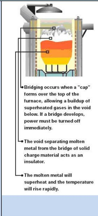
Superheating which occurs very rapidly in an induction furnace can result in refractory failure due to two main reasons:
