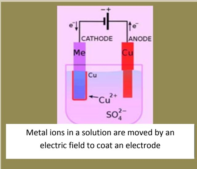
This deposition bestows certain desired properties such as abrasion & wear resistance, corrosion protection, aesthetic appearance, etc. which the surface otherwise lacks. It is also used to build up thickness on undersized parts.
